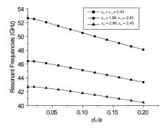
Figure 6. Resonant frequency versus the substrate thickness for: Isotropic ( $\varepsilon_{1x} = \varepsilon_{1z} = 2.43$ ); positive uniaxial ( $\varepsilon_{1x} = 2.43$ ,  $\varepsilon_{1z} = 2.88$ ); and negative uniaxial ( $\varepsilon_{1x} = 2.43$ ,  $\varepsilon_{1z} = 1.88$ ),  $T/T_c =$ 0.5,  $t = 0.15 \,\mu\text{m}$ ,  $\sigma = 210 \,\text{s/mm}$ ,  $\lambda_0 = 1500 \,\text{\AA}$ ,  $a = 1.5 \,\text{mm}$ .
