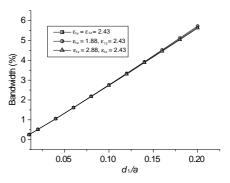
Figure 5. Bandwidth versus the substrate thickness for: Isotropic ( $\varepsilon_{1x} = \varepsilon_{1z} = 2.43$ ); positive uniaxial ( $\varepsilon_{1x} = 1.88, \varepsilon_{1z} = 2.43$ ), negative uniaxial ( $\varepsilon_{1x} = 2.88, \varepsilon_{1z} = 2.43$ ),  $T/T_c = 0.5, t = 0.15 \,\mu\text{m}, \sigma = 210 \,\text{s/mm}, \lambda_0 = 1500 \,\text{\AA}, a = 1.5 \,\text{mm}.$
