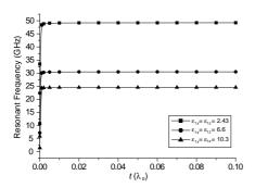
Figure 2. The resonant frequency versus the thickness of patch ( $\sigma_n = 210 \text{ s/mm}$ ,  $\lambda_0 = 1500 \text{ Å}$  and  $T/T_c = 0.5$ , a = 1 mm,  $d_1 = 1.2 \text{ mm}$ ).
