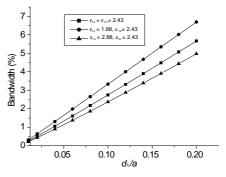
Figure 7. Bandwidth versus the substrate thickness for: Isotropic ( $\varepsilon_{1x} = \varepsilon_{1z} = 2.43$ ); positive uniaxial ( $\varepsilon_{1x} = 2.43$ ,  $\varepsilon_{1z} = 2.88$ ); and negative uniaxial ( $\varepsilon_{1x} = 2.43$ ,  $\varepsilon_{1z} = 1.88$ ),  $T/T_c = 0.5$ ,  $t = 0.15 \,\mu\text{m}$ ,  $\sigma = 210 \,\text{s/mm}$ ,  $\lambda_0 = 1500 \,\text{\AA}$ ,  $a = 1.5 \,\text{mm}$ .
