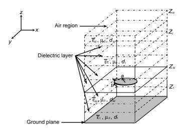
Superconducting circular microstrip antenna with Figure 1. multilayered configuration and anisotropic dielectrics.
