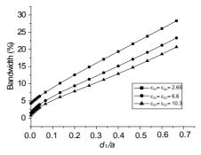
Figure 9. Bandwidth versus the air separation, for circular microstrip antenna for three dielectric constant:  $\varepsilon_{2x} = \varepsilon_{2z} = 2.65$ ,  $\varepsilon_{2x} = \varepsilon_{2z} = 6.6$ , and  $\varepsilon_{2x} = \varepsilon_{2z} = 10.3$ , a = 1.5 mm.  $\sigma_n = 210$  s/mm,  $\lambda_0 = 1500$  Å, and  $T/T_c = 0.5$ , and t = 0.02 µm.
