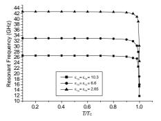
Figure 3. The resonant frequency versus the normalized temperature ( $\sigma_n = 210 \text{ s/mm}$ ,  $\lambda_0 = 1500 \text{ Å}$  and  $t_c = 89^\circ$ , a = 1 mm,  $d_1 = 1.2 \text{ mm}$  and t = 0.02 µm).
