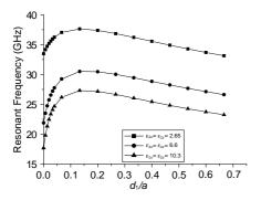
Figure 8. Resonant frequency versus the air separation, for circular microstrip antenna for three dielectric constant:  $\varepsilon_{2x} =$  $\varepsilon_{2z} = 2.65$ ,  $\varepsilon_{2x} = \varepsilon_{2z} = 6.6$ , and  $\varepsilon_{2x} = \varepsilon_{2z} = 10.3$ , a = 1.5 mm.  $\sigma_n = 210$  s/mm,  $\lambda_0 = 1500$  Å, and  $T/T_c = 0.5$ , and t = 0.02 µm.
