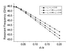
Figure 4. Resonant frequency versus the substrate thickness for: Isotropic ( $\varepsilon_{1x} = \varepsilon_{1z} = 2.43$ ); positive uniaxial ( $\varepsilon_{1x} = 1.88$ ,  $\varepsilon_{1z} = 2.43$ ), negative uniaxial ( $\varepsilon_{1x} = 2.88$ ,  $\varepsilon_{1z} = 2.43$ ),  $T/T_c =$ 0.5,  $t = 0.15 \,\mu\text{m}$ ,  $\sigma = 210 \,\text{s/mm}$ ,  $\lambda_0 = 1500 \,\text{\AA}$ ,  $a = 1.5 \,\text{mm}$ .
