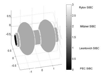
Figure 2. Piecewise surface impedance boundary conditions.
