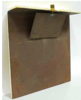
Figure 2. The photograph of constructed prototype of the proposed patch antenna ( \alpha = 30^\circ ) with an inclined patch for generating a downtilt main beam.
