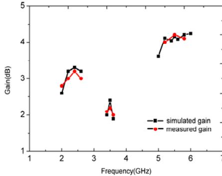
**Figure 11.** Simulated and measured gain of proposed antenna.
