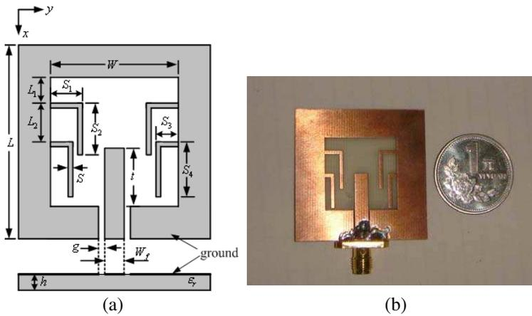
**Figure 1.** Geometry and photograph of the proposed antenna.
