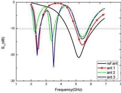
**Figure 3.**  $S_{11}$  of the reference antenna and antenna 1, antenna 2 and antenna 3.
