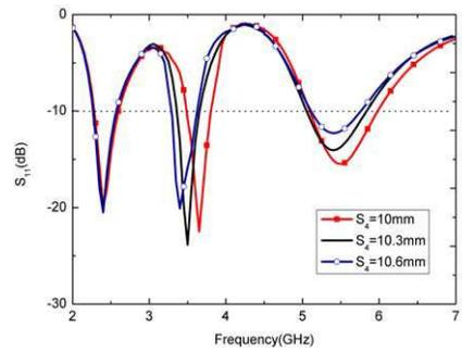
**Figure 7.** Simulated  $S_{11}$  of proposed antenna as the function of frequency with the variation in  $S_4$ .
