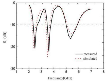
**Figure 4.** Simulated and measured  $S_{11}$  of proposed antenna.
