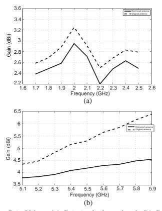
Figure 6. Gain Values; (a) Gain in the lower band; (b) Gain in the upper band.
