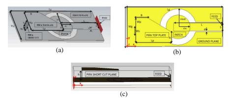
**Figure 1.** Antenna configuration. (a) Complete antenna; (b) Top view; (c) Front view.
