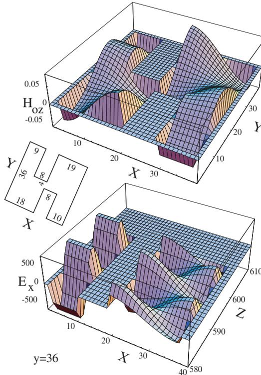
**Figure 2.**  $H_{oz}$  pattern of the 9th TE mode for a ridged rectangular waveguide (top). Geometry of this guide (middle). Propagation along the  $Z$ -axis of the  $E_x$  component of the 9th mode, at  $y = 38$  cells (bottom). All dimensions are in cells ( $\Delta x = \Delta y = 333.3 \text{ mm}$ ,  $\Delta z = 9.0 \text{ mm}$ ,  $\Delta t = 29.70 \text{ ps}$ ).
