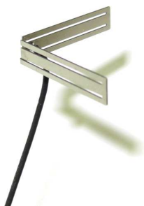
Figure 2. Photo of a constructed prototype made of a 0.3-mm thick alloy and fed by a 50\text{-}\Omega mini-coaxial cable.
