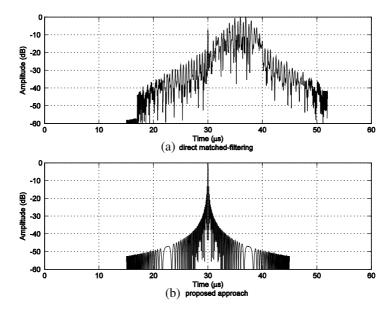
**Figure 5.** Cancelation of C&I jamming using transmission pulse block II.
