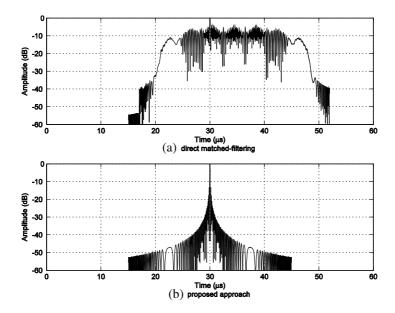
Figure 6. Cancelation of SMSP jamming using transmission pulse block II.
