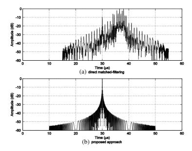
Figure 3. Cancelation of C&I jamming using transmission pulse block I.
