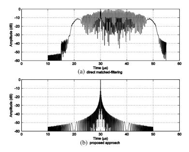
Figure 4. Cancelation of SMSP jamming using transmission pulse block I.
