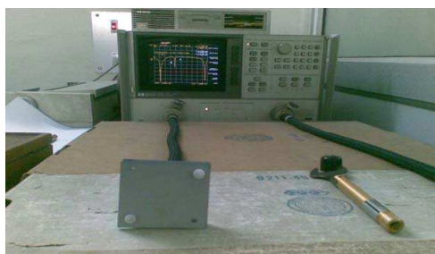
Figure 11. The fabricated antenna being tested on a network analyzer.
