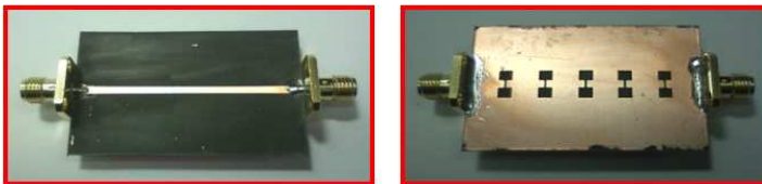
Figure 10. Fabricated microstrip line with DGS.
