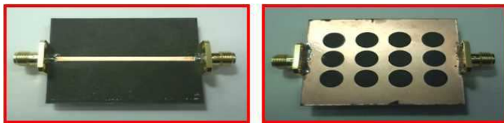
Figure 13. Fabricated microstrip line with PBG.
