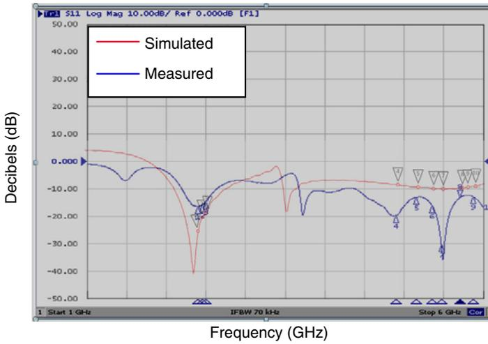
Figure 6. Comparison between simulated and measured return loss.
