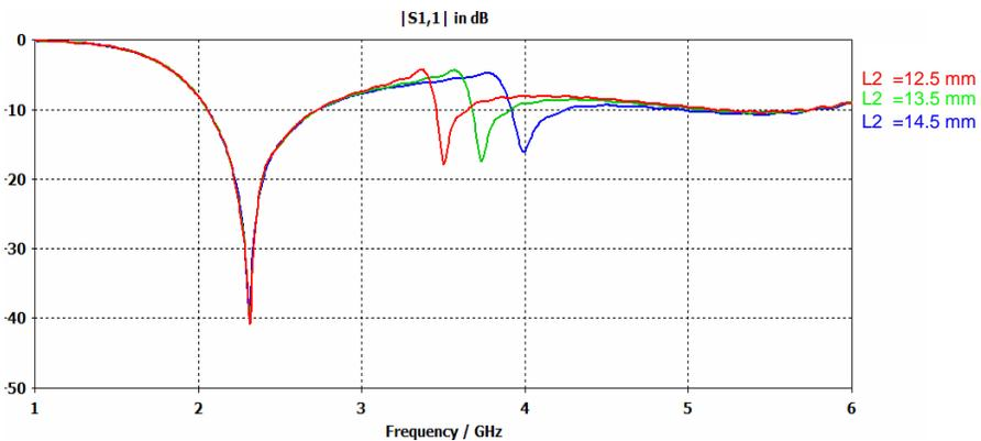
**Figure 4.** Simulated return loss of the radiating element for various  $L_2$ .
