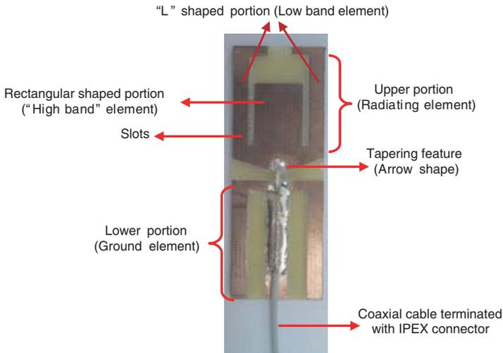
**Figure 1.** The proposed antenna design.
