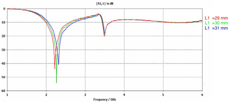
**Figure 3.** Simulated return loss of the radiating element for various  $L_1$ .
