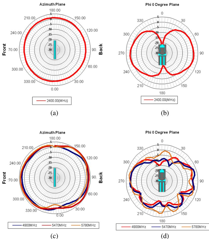
**Figure 11.** For 2450 MHz (low band). (a) Azimuth radiation pattern. (b) Elevation 0° radiation pattern; for 4900–5780 MHz (high band). (c) Azimuth radiation pattern. (d) Elevation 0° radiation pattern.
