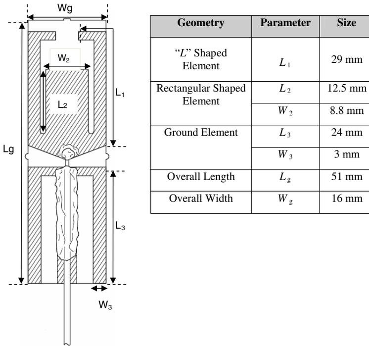
**Figure 2.** Geometry and dimension of the proposed antenna.
