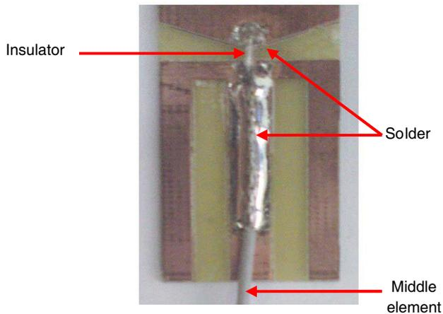
**Figure 5.** Feeding technique on the ground element.
