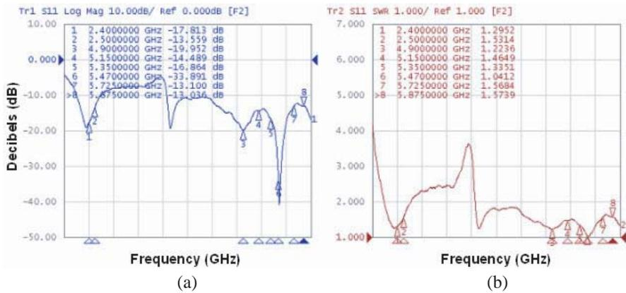
Figure 8. (a) Return loss  $S_{11}$  and (b) measured VSWR.
