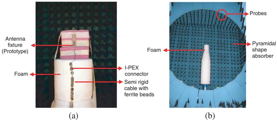
**Figure 10.** (a) Inside view of the 3D chamber and (b) test method.
