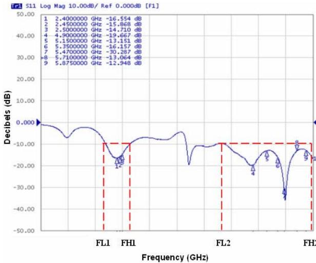
Figure 7. Bandwidth calculation.
