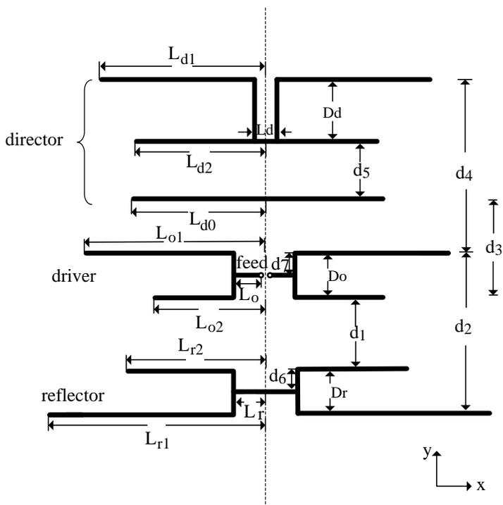
**Figure 1.** Configuration of the proposed antenna.
