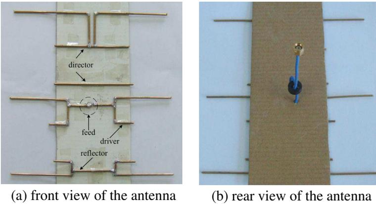
**Figure 3.** Fabricated dual-band Yagi antenna, (a) is the front of the antenna and (b) is the back of the antenna.
