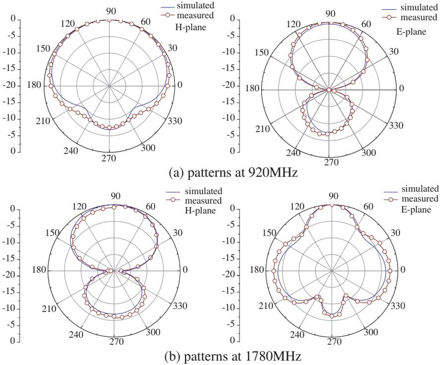
**Figure 5.** Simulated and measured radiation patterns in  $E$ -plane and  $H$ -plane at the frequencies 920 MHz and 1780 MHz, (a) for 920 MHz, and (b) for 1780 MHz.
