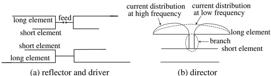
**Figure 2.** Explanation for each part of the proposed antenna, (a) for the reflector and driver, and (b) for the director.
