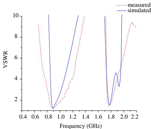
**Figure 4.** Simulated and measured VSWR of the proposed antenna.
