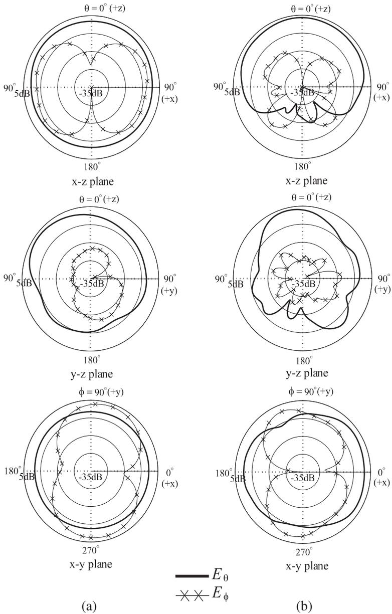
**Figure 6.** Measured radiation patterns for the proposed antenna in Fig. 2 at (a) 2.45 GHz, (b) 5.5 GHz.
