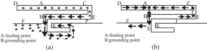
**Figure 4.** Simulated surface current distributions for case 2 in Fig. 2 at (a) 2.8 GHz, (b) 5.5 GHz.
