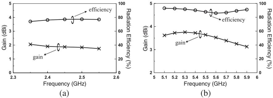
**Figure 7.** Measured maximum boresight antenna gain and radiation efficiency against for the proposed antenna in Fig. 2.
