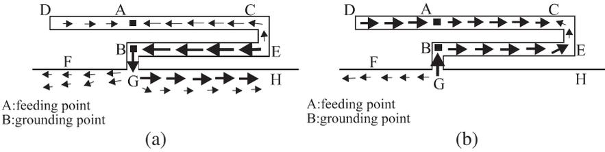
**Figure 3.** Simulated surface current distributions for case 1 in Fig. 2 at (a) 3.4 GHz, (b) 5.5 GHz.
