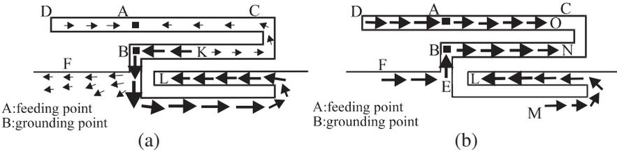
**Figure 5.** Simulated surface current distributions for case 3 (proposed) in Fig. 2 at (a) 2.45 GHz, (b) 5.5 GHz.
