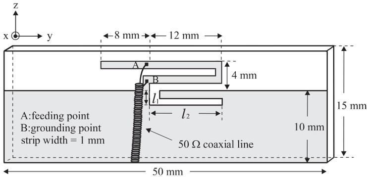
**Figure 1.** Geometry of the proposed folded antenna for WLAN application.
