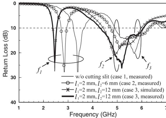
**Figure 2.** Measured and simulated return loss against frequency for the folded antenna with different cutting slot length.
