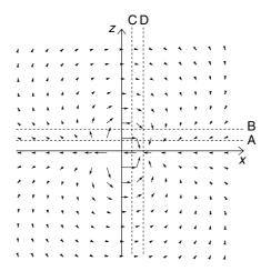
**Figure 2.** Magnetic dipole moment centered at (x; z) = (0; 0) using Eqs. (5) and (6). The four dashed lines are indexed A, B, C and D. See text for more info.
