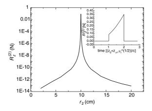
**Figure 6.** Numerical instantaneous resultant  $R_z^{(2)}$  vs. receptors radius  $r_2$ , for an emitter-receptor distance  $z_0 = 0.1 \text{ mm}$  and an emitter radius  $r_1 = 10 \text{ cm}$ . The inset of Fig. 3 shows a full period of the calculated thrust  $R_z^{(2)}$  versus time with  $r_1 = r_2 = 10 \text{ cm}$ ,  $L_2 = 10 \text{ mH}$ ,  $z_{\mu r} = 10 \text{ cm}$  and  $N_s = 140$ .
