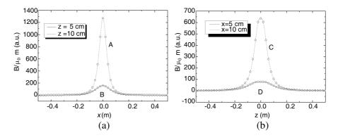
**Figure 3.** Rescaled magnetic field  $\sqrt{B_x^2 + B_z^2}/\mu_0 m$  calculated (symbols) with Eqs. (5) and (6) under dipole approximation  $|\vec{R}| \gg r$  versus the rescaled analytical expressions (dashed lines and lines). The rescaled magnetic fields are calculated along the (a) x axis and (b) z axis along two axes separating the centre (5 and 10 cm).
