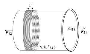
Figure 4. Cylindrical magnetic core placed inside the emitter coil. The receptor ring is placed outside the magnetic core. See text for more info.
