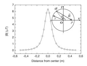
**Figure 1.** Continuous line: norm of magnetic field along z axis according to the known Biot-Savart equation for a ring radius r = 10 cm and a current i = 1 A. Empty circles: norm of magnetic field using Eq. (6) with the same parameters and with  $B_z = \lim_{\rho \to 0} B_z(\rho, z, t)$ . The inset shows the ring in the (Oxy) plane, the cylindrical coordinates  $(z, \theta, \rho)$ , the ring radius r and the observation point  $\vec{R}$ .
