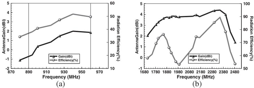
**Figure 9.** Measured gain and radiation efficiency of the proposed antenna at (a) 880–960 MHz and (b) 1710–2484 MHz.
