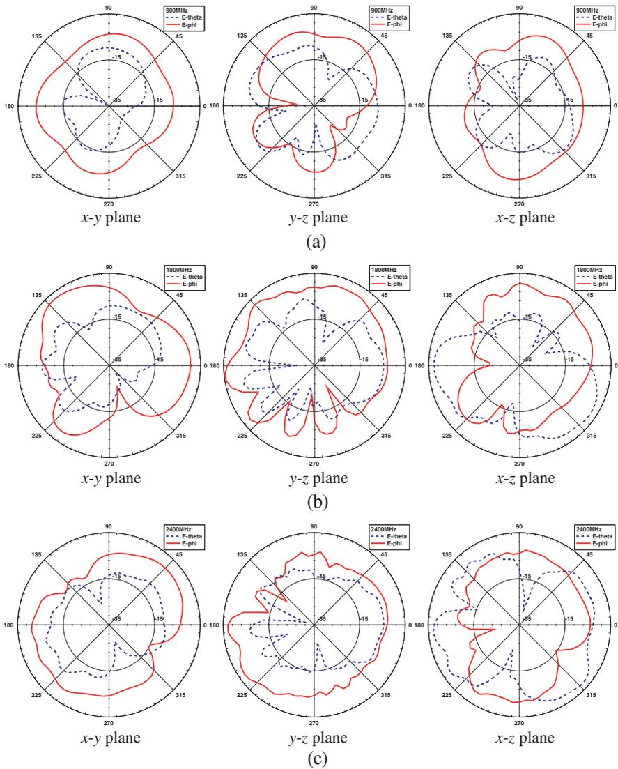
**Figure 8.** Measured radiation patterns of the proposed antenna at (a) 900 MHz, (b) 1800 MHz, and (c) 2400 MHz.
