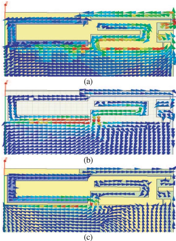
**Figure 7.** Current distributions of the proposed antenna at (a) 920 MHz, (b) 1710 MHz, and (c) 2350 MHz.
