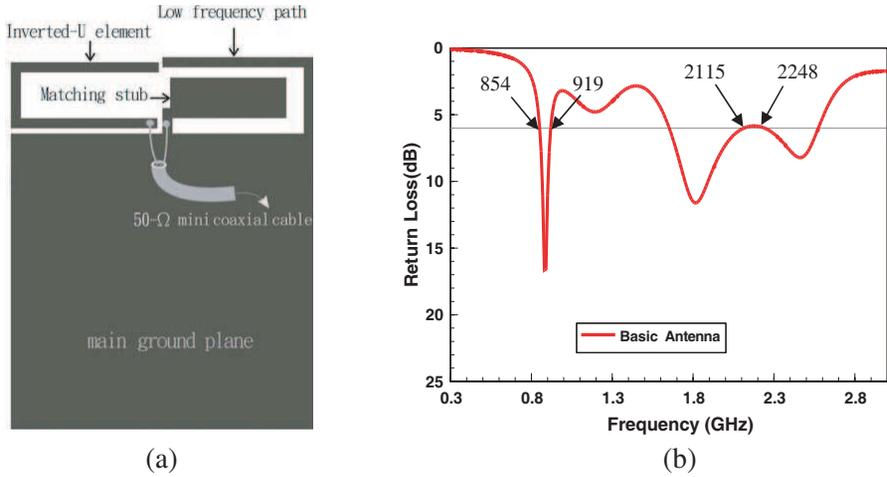
**Figure 1.** (a) Basic antenna structure. (b) Simulated return loss of basic antenna.
