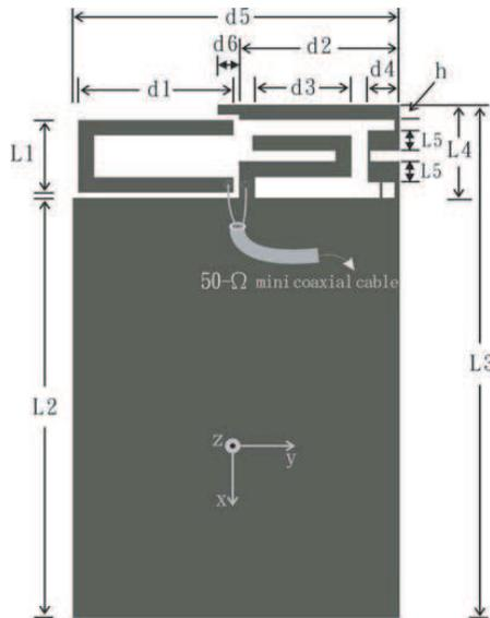
**Figure 2.** Structure of the proposed antenna.
