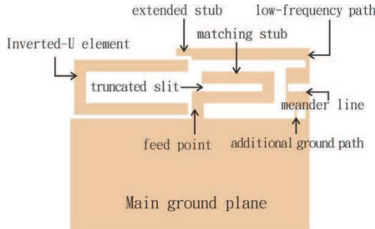
**Figure 3.** Elements of the proposed antenna.
