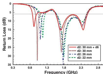
**Figure 6.** Simulated return losses for different lengths of  $d_2$ .
