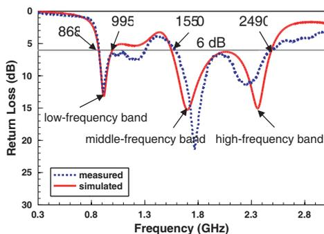
**Figure 4.** Simulated and measured return loss of the proposed antenna.
