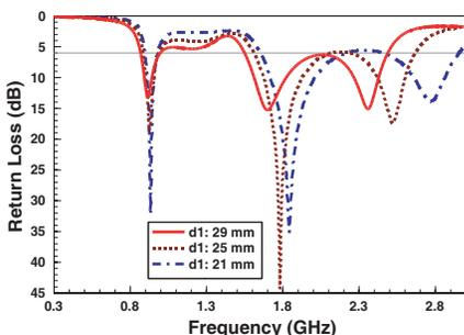
**Figure 5.** Simulated return losses for different lengths of  $d_1$ .
