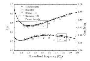
**Figure 9.** Normalized aperture admittance of the open-ended WR-90 waveguide with an infinite flange.
