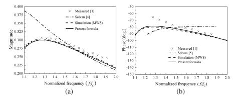
Figure 2. Aperture reflection coefficient at the open-end of the standard WR-90 waveguide without a flange. (a) Magnitude, and (b) phase.
