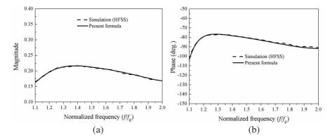
Figure 8. Aperture reflection coecient of the open-ended WR-34 waveguide with an infinite flange. (a) Magnitude, and (b) phase.
