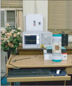
Figure 14. Snapshot of S_{11} measurement set up.
