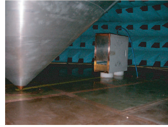
Figure 4. The conical antenna and the computer box in the anechoic chamber (CE-SAME equipment).
