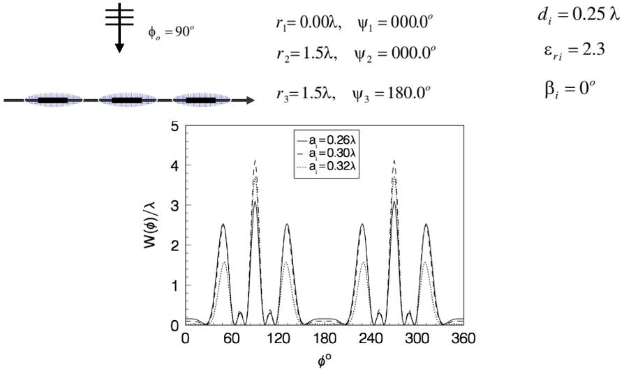
**Figure 6.** Echo width pattern for different dielectric thickness.
