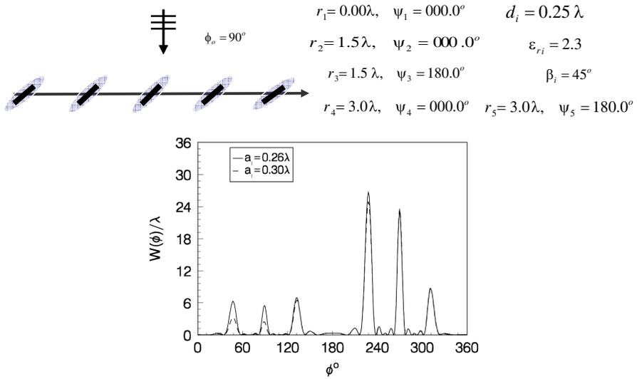
Figure 9. Echo width pattern for different dielectric thickness.
