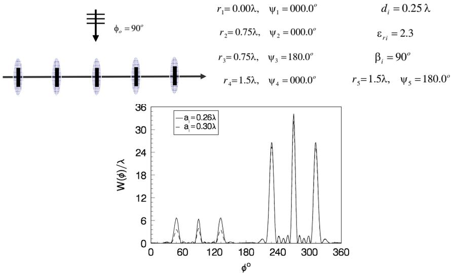
Figure 10. Echo width pattern for different dielectric thickness.
