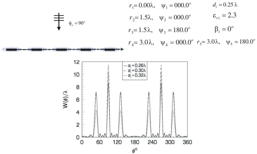
**Figure 8.** Echo width pattern for different dielectric thickness.
