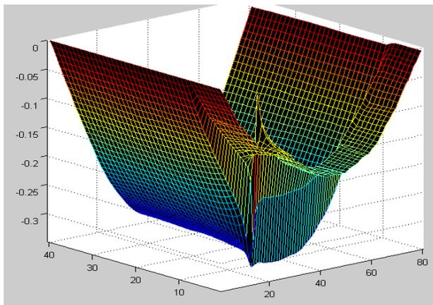
**Figure 10.** Field distribution on the transverse section of the first higher mode's  $E_x$ -component when  $\varepsilon_r = 1.5$ .
