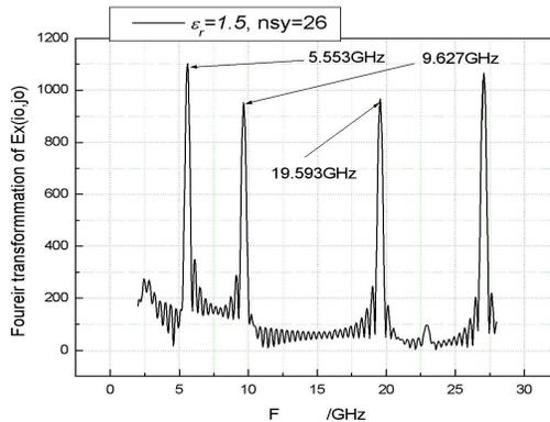
**Figure 2.** The cutoff frequencies of the PRWG, in which  $\epsilon_r = 1.5$ ,  $nsy = 26$ ,  $a = 15 \text{ mm}$ ,  $b = 7 \text{ mm}$ ,  $h = 1.4 \text{ mm}$ . The sample point's coordinates are  $io \times dx, jo \times dy$  ( $io = 11, jo = 24, dx = 7 \text{ mm}/40, dy = 15 \text{ mm}/80$ ).
