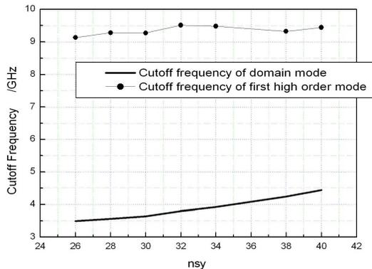
**Figure 4.** Cutoff frequencies for the lowest two modes of the PRWG when  $nsy$  is changed. Here the width of the metal plane is equal to  $(a - nsy * dy)$ .
