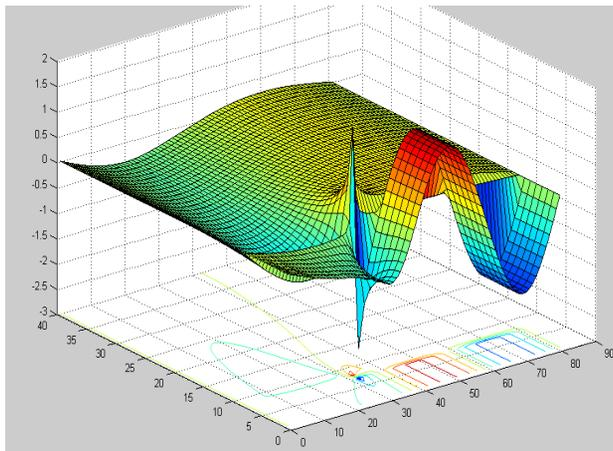
**Figure 14.** Field distribution on the transverse section of the second higher mode's  $E_x$ -component, when  $\epsilon_r = 4.3$ .
