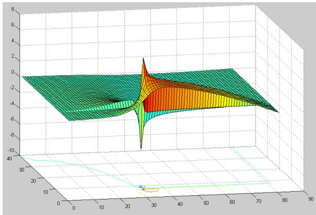
**Figure 12.** Field distribution on the transverse section of the dominant mode's  $E_x$ -component when  $\varepsilon_r = 4.3$ .
