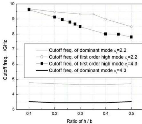
Figure 8. Cutoff frequencies of the lowest modes when the ratio of wide side to narrow side is changed.
