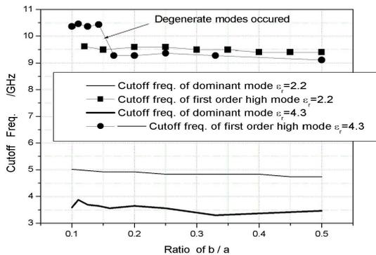
**Figure 6.** Cutoff frequencies of the lowest modes when the ratio of wide side to narrow side is changed.
