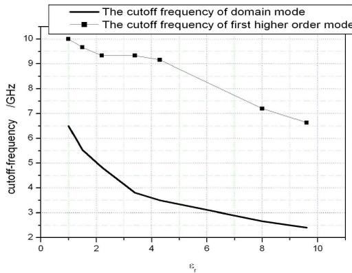
**Figure 3.** Cutoff frequencies for the lowest two modes of the PRWG when relative permittivity of the dielectric layer is changed.
