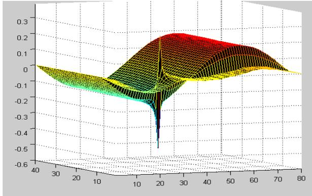
**Figure 11.** Field distribution on the transverse section of the second higher mode's  $E_x$ -component, when  $\varepsilon_r = 1.5$ .
