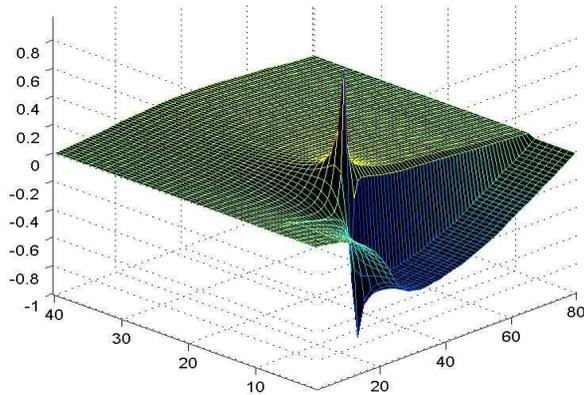
**Figure 9.** Field distribution on the transverse section of the dominant mode's  $E_x$ -component when  $\varepsilon_r = 1.5$ .
