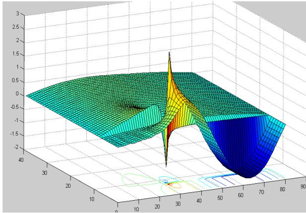
**Figure 13.** Field distribution on the transverse section of the first higher mode's  $E_x$ -component when  $\epsilon_r = 4.3$ .
