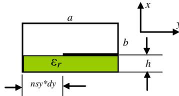
**Figure 1.** The planar rectangular waveguide loaded with dielectric layer. The metal plane's width equals  $a - nsy * dy$ .  $dy$  is the space step in  $y$ -direction. The thickness of the dielectric layer is  $h$ .
