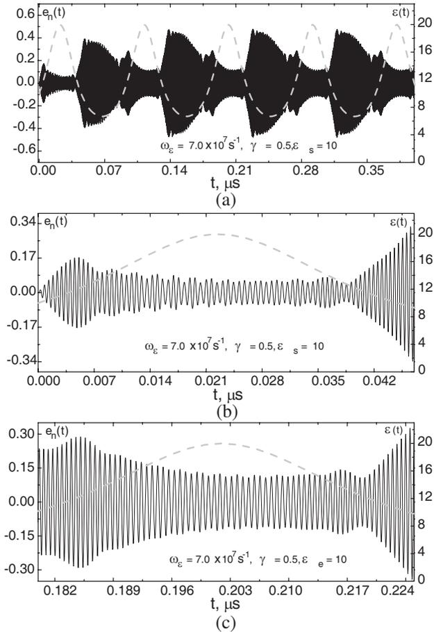
**Figure 7.** Solenoidal mode amplitude of electric field strength (solid line), permittivity (dotted line).  $A = 10^9$ ,  $k_n/2\pi = 10.599$  GHz,  $\omega_n/2\pi = 1.935$  GHz,  $\sigma/2\epsilon_0\epsilon_s = 2 \times 10^7 s^{-1}$ .
