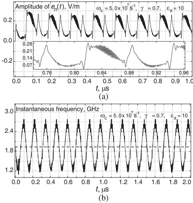
**Figure 10.** (a) Envelope amplitude and (b) instantaneous frequency of solenoidal mode amplitude of electric field strength.  $A = 10^9$ ,  $k_n/2\pi = 10.599$  GHz,  $\omega_n/2\pi = 1.935$  GHz,  $\sigma/2\varepsilon_0\varepsilon_s = 2 \times 10^7$  s $^{-1}$ .
