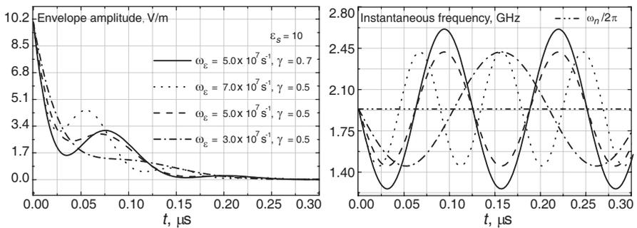
Figure 6. Time dependence of envelope amplitude and instantaneous frequency of  $e_n(t)$ .  $e_n^0 = 10$ ,  $k_n/2\pi = 10.599$  GHz,  $\omega_n/2\pi = 1.935$  GHz,  $\sigma/2\varepsilon_0\varepsilon_s = 2 \times 10^7$  s<sup>-1</sup>.
