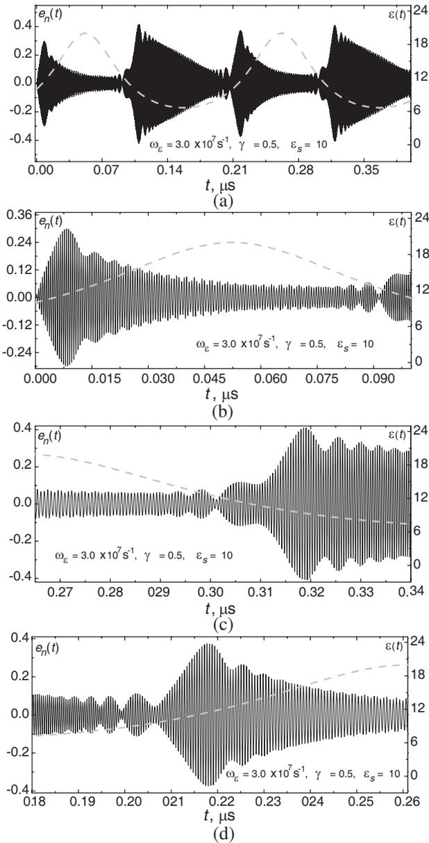
**Figure 9.** Solenoidal mode amplitude of electric field strength (solid line), permittivity (dotted line).  $A = 10^9$ ,  $k_n/2\pi = 10.599 \text{ GHz}$ ,  $\omega_n/2\pi = 1.935 \text{ GHz}$ ,  $\sigma/2\epsilon_0\epsilon_s = 2 \times 10^7 \text{ s}^{-1}$ .
