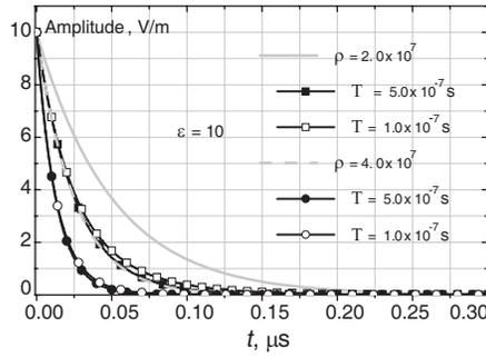
**Figure 12.** Time-dependence of free oscillations.
