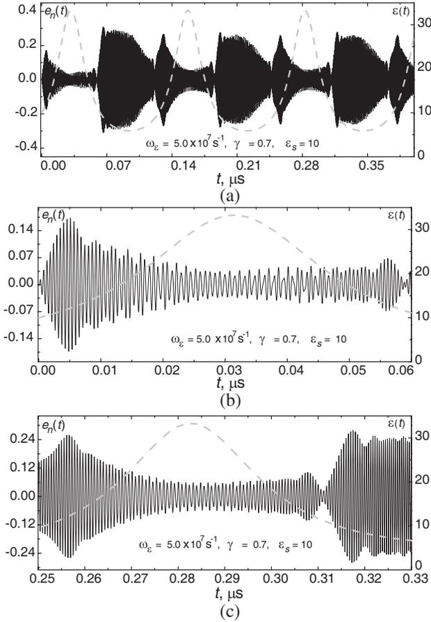
**Figure 8.** Solenoidal mode amplitude of electric field strength (solid line), permittivity (dotted line).  $A = 10^9$ ,  $k_n/2\pi = 10.599 \text{ GHz}$ ,  $\omega_n/2\pi = 1.935 \text{ GHz}$ ,  $\sigma/2\varepsilon_0\varepsilon_s = 2 \times 10^7 \text{ s}^{-1}$ .
