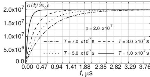
**Figure 11.** Time dependence of medium conductivity.
