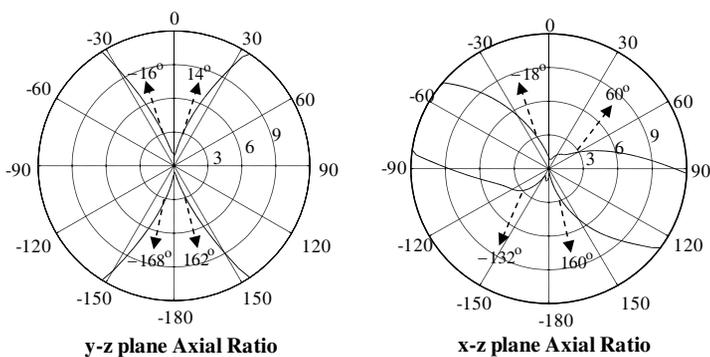
**Figure 4.** Simulated axial ratios of the proposed wide strip dipole antenna at 1.94 GHz.
