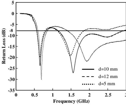
**Figure 13.** Simulated return loss for different port length  $d$ .
