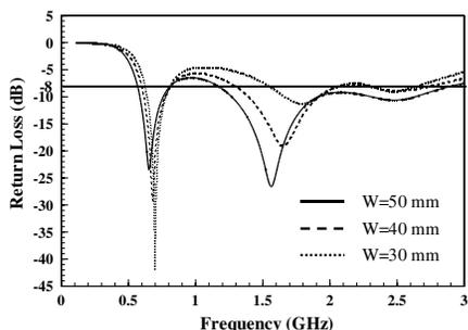
**Figure 9.** Simulated return loss for different slab width  $W$ .
