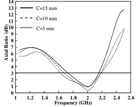
**Figure 12.** Simulated axial ratios for different overlapped square width  $C$ .
