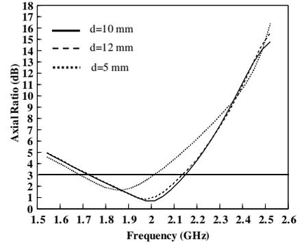
**Figure 14.** Simulated axial ratios for different port length  $d$ .
