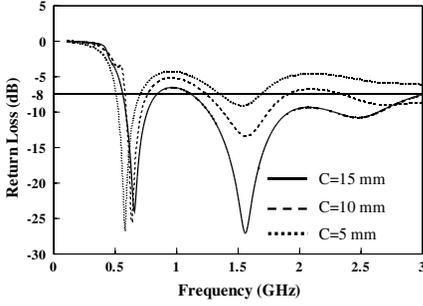
**Figure 11.** Simulated return loss for different overlapped square width  $C$ .
