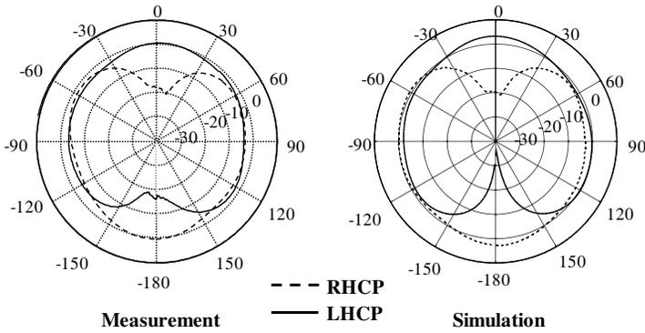
**Figure 5.** Measured and simulated  $y$ - $z$  plane radiation patterns of the proposed wide strip dipole antenna at 1.94 GHz.
