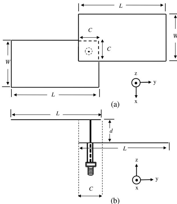
**Figure 1.** Geometrical configuration of a wideband wide-strip dipole antenna for circularly polarized wave operations: (a) Top view; (b) side view.
