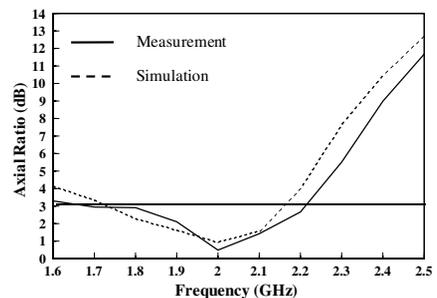
**Figure 3.** Measured and simulated axial ratios of the proposed wide strip dipole antenna with the same parameters in Fig. 2.
