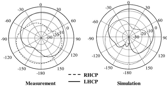
**Figure 6.** Measured and simulated  $x$ - $z$  plane radiation patterns of the proposed wide strip dipole antenna.
