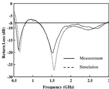
**Figure 2.** Measured and simulated return loss of the proposed wide strip dipole antenna with parameters:  $L = 100$  mm,  $W = 50$  mm,  $d = 10$  mm, and  $C = 15$  mm.
