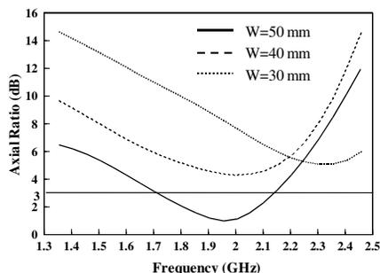
**Figure 10.** Simulated axial ratios for different slab width  $W$ .
