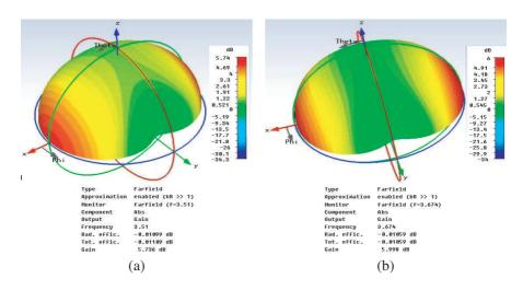
Figure 11. Radiation patterns (3D Views) of FRC-1 DRAs with  $\varepsilon_r = 8$ . (a) Conventional FRC DRA. (b) Modified FRC-1 DRA.
