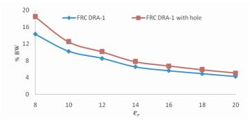
**Figure 8.** Effect of material dielectric constant on percentage return loss bandwidth of conventional and modified FRC-1 DRAs.
