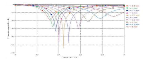
Figure 9. Effect of cylindrical hole diameter on return loss vs. frequency characteristics of modified FRC-1 DRA with  $\varepsilon_r = 20$ .
