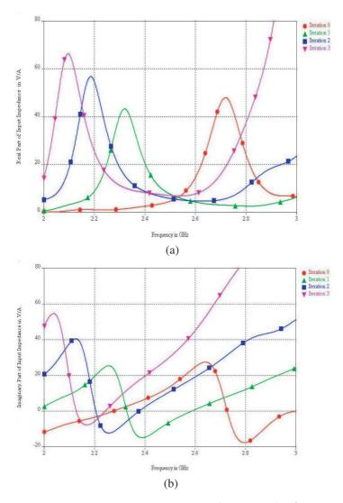
Figure 5. Variation in input impedance with frequency for conventional FRC DRAs. (a) Real part. (b) Imaginary part.
