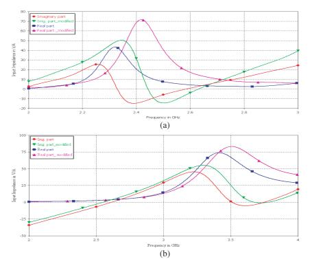
Figure 10. Variation of input impedance with frequency for conventional FRC-1 DRA and modified FRC-1 DRA. (a) with  $\varepsilon_r = 20$ , (b) with  $\varepsilon_r = 8$ .
