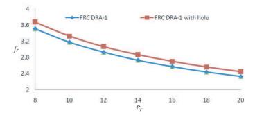
**Figure 7.** Effect of material dielectric constant on resonant frequency of conventional and modified FRC-1 DRAs.
