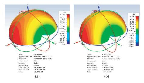
Figure 12. Radiation patterns (3D Views) of FRC-1 DRAs with  $\varepsilon_r = 20$ . (a) Conventional FRC DRA. (b) Modified FRC-1 DRA.
