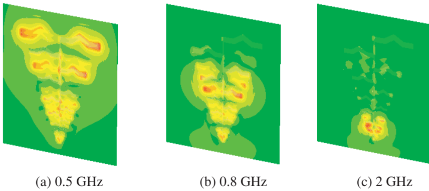
Figure 4. Current distribution of 1st iteration antenna.
