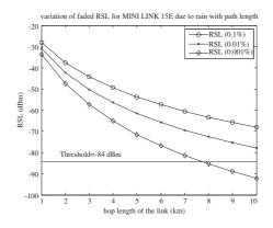
**Figure 2.** Rain fade margins for different path lengths at MINI-LINK 15E.
