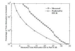
Figure 7. Rain attenuation distribution measured at 23 GHz frequency over microwave links at Kuala Lumpur -2 and those predicted by ITU-R.
