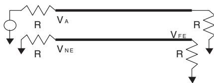
Figure 3. Parallel transmission lines with matched terminations. A pulse transmitted on the upper line generates cross-talk on the lower line that propagates in a manner equivalent to the case of the serpentine line segment shown in Fig. 2.
