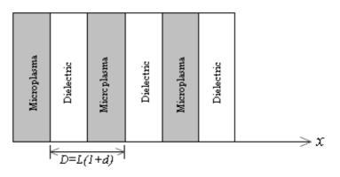
Figure 1. Periodic variation of plasma and dielectric showing 1-D plasma photonic crystals.
