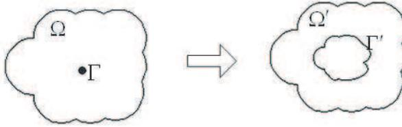
**Figure 1.** Illustration of the coordinate transformation for an arbitrary cloak.
