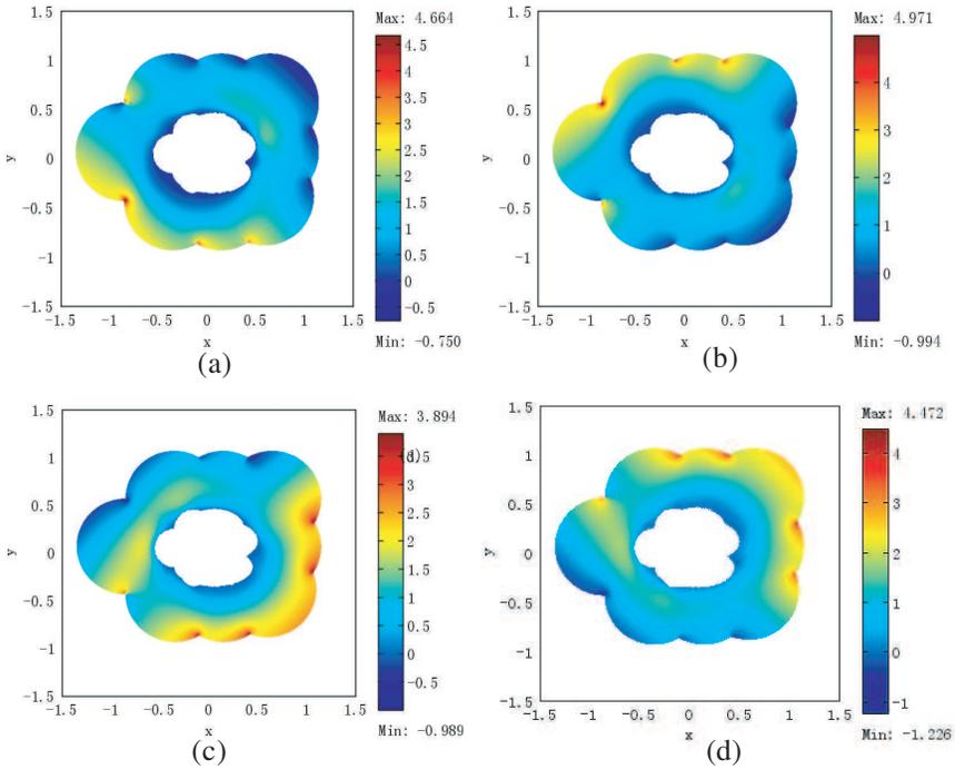
**Figure 3.** The contour plots of relative permittivity  $\varepsilon_{zz}$  determined by different Poisson's equations with factor function (a)  $f_x = f_y = 4$ , (b)  $f_x = 4$ ,  $f_y = -4$ , (c)  $f_x = -4$ ,  $f_y = 4$  and (d)  $f_x = f_y = -4$ .
