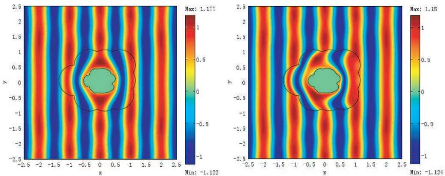
**Figure 4.** The contour plots of the electric fields determined by different kinds of Poisson's equations with (a)  $f_x = f_y = 0$  and (b)  $f_x = 4$ ,  $f_y = -4$ .
