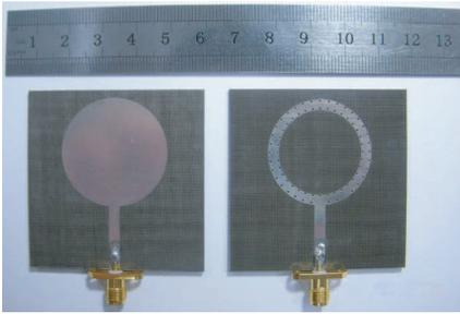
**Figure 3.** Pictures of the reference and proposed antennas.
