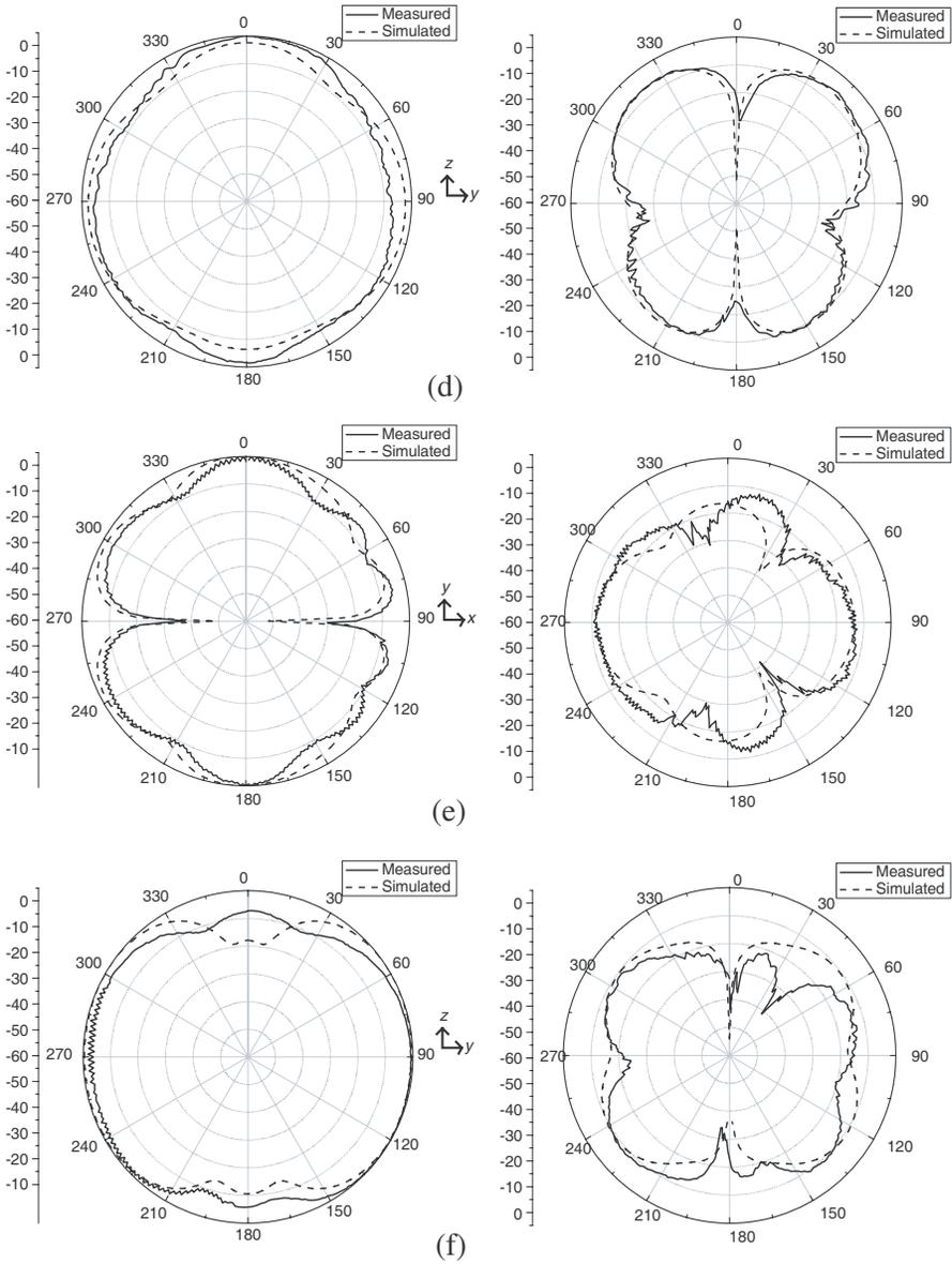
**Figure 7.** Co- and cross-polar radiation pattern at (a) 3.0 GHz in *E*-plane, (b) 3.0 GHz in *H*-plane, (c) 6.0 GHz in *E*-plane, (d) 6.0 GHz in *H*-plane, (e) 9.0 GHz in *E*-plane, (f) 9.0 GHz in *H*-plane.
