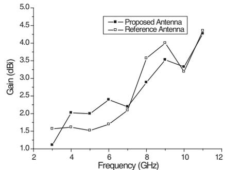
**Figure 6.** Gain curves of the reference antenna and proposed antenna.
