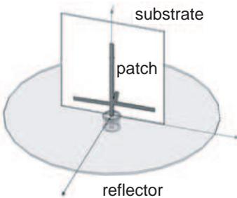
**Figure 2.** The configuration of the tree-shaped antenna.
