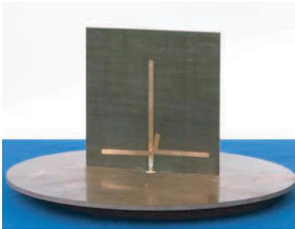
**Figure 4.** The optimized structure of the antenna.
