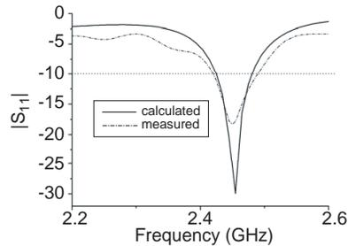
**Figure 5.** The measured and simulated  $S_{11}$  of the antenna.
