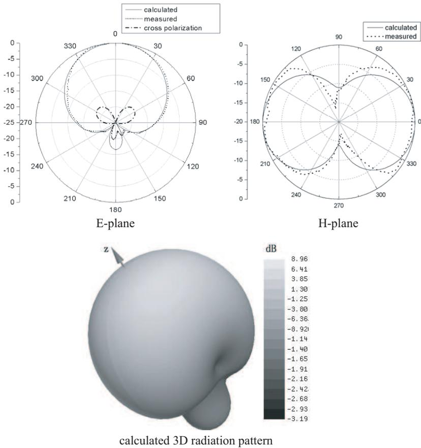
**Figure 6.** The calculated and measured radiation pattern at 2.45 GHz.
