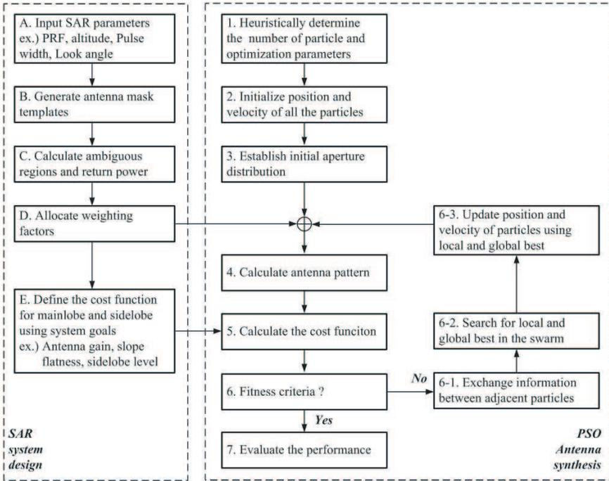
**Figure 2.** Design flow diagram for the SAR performance evaluation based on PSO. The PSO technique is applied to the SAR system design. For optimization of the cost function, the mask pattern and weighting factors are calculated with respect to the SAR parameters.
