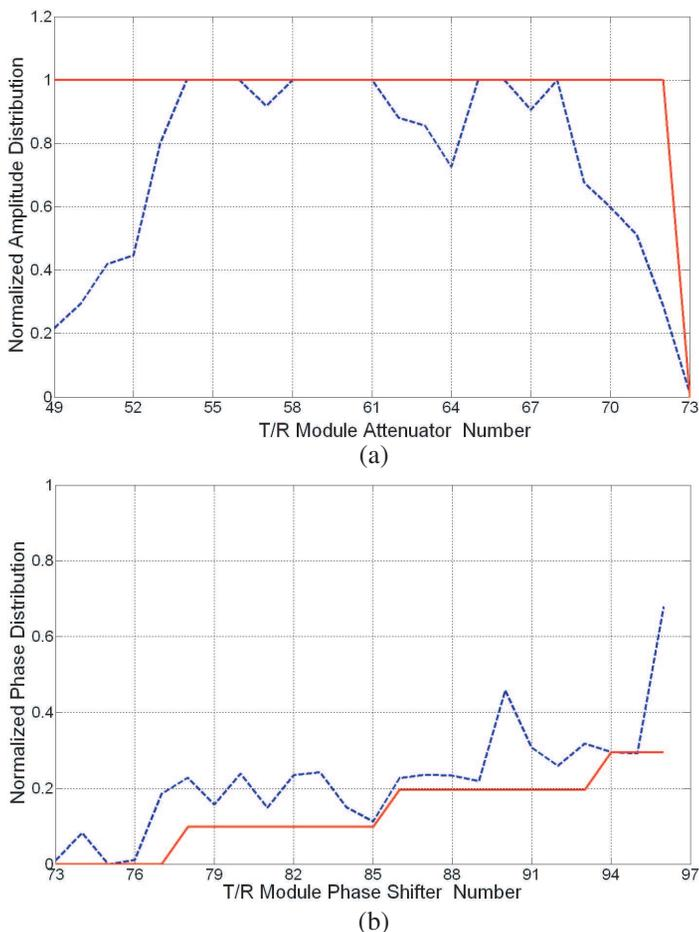
**Figure 4.** T/R module's excitation coefficients optimized by PSO after 150 iterations. (a) Normalized amplitude distribution and (b) normalized phase distribution (solid line: Initial amplitude and phase distribution; dashed line: Optimized amplitude and phase distribution).
