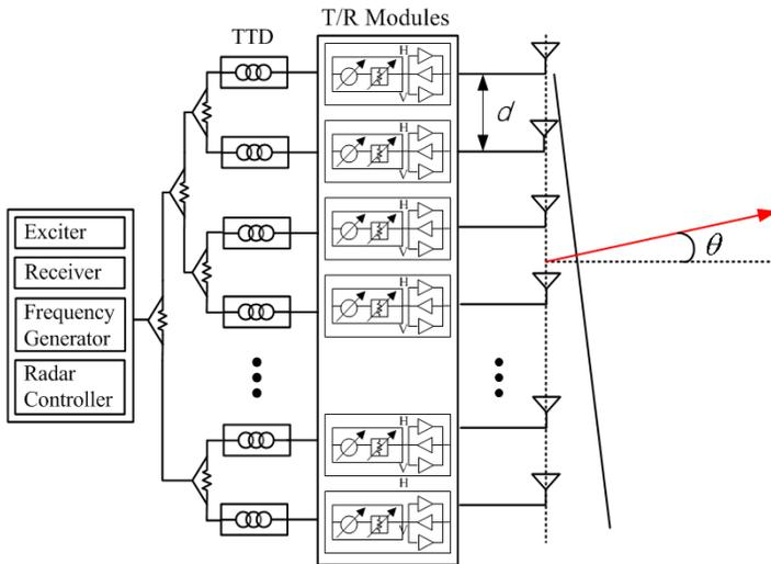
**Figure 1.** Active phased array SAR configuration. The radiating elements are composed of the slot coupled microstrip patch antenna. Each T/R module provides (H/V) horizontal and vertical polarizations. The true time delay (TTD) can stabilize the antenna pattern in relation to the frequency bandwidth.
