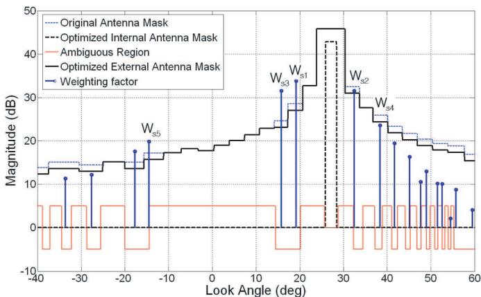
**Figure 3.** Antenna mask and adaptive weighting factors selected at the ambiguous regions in proportion to the return power based on Table 1. The shaded areas indicate the ambiguous region defined from the radar parameters.
