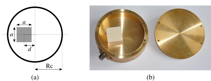
Figure 8. Circular cavity resonator loaded with single square dielectric post: (a) Schematic view, (b) photo of the fabricated structure.
