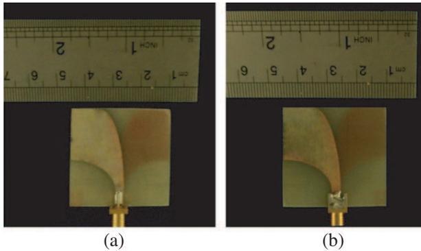
**Figure 4.** Photograph of the fabricated antenna (a) top layer, (b) bottom layer.
