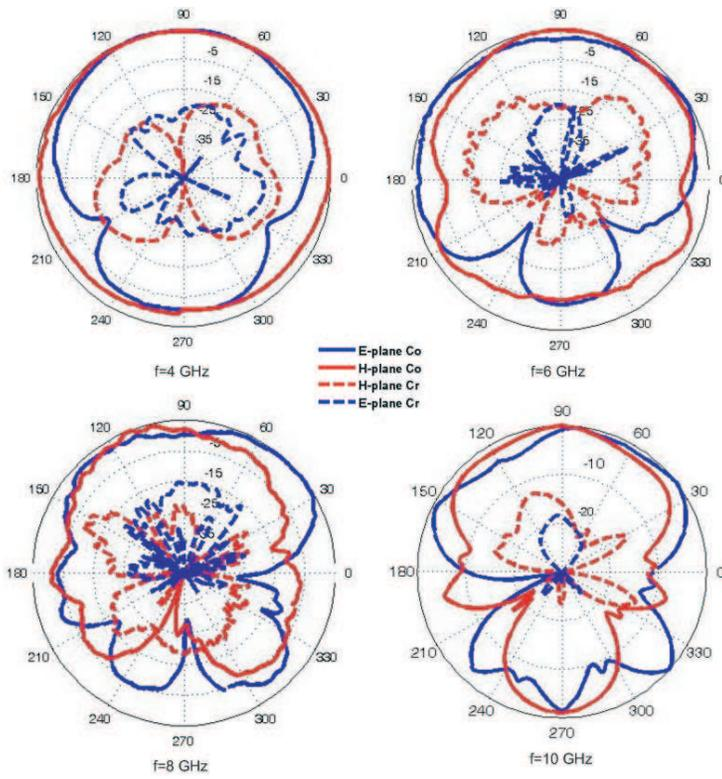
**Figure 7.** Measured radiation patterns of the proposed antenna at 4, 6, 8 and 10 GHz.
