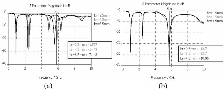
**Figure 5.** The simulated return loss with different values of  $br$  (a) straight dipole and (b) meandered dipole.
