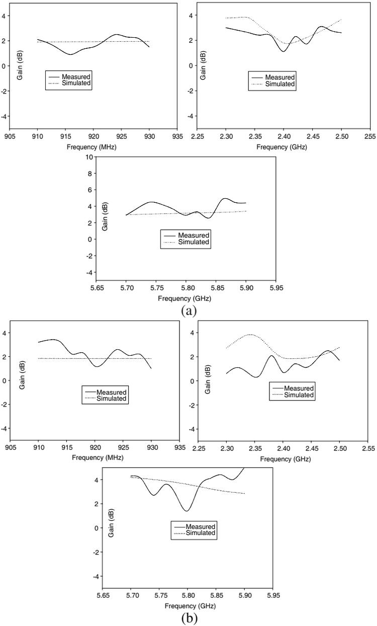
**Figure 6.** The simulated and measured gain of triple-band printed dipole antenna (a) straight and (b) meandered.
