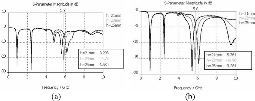
**Figure 4.** The simulated return loss with different values of  $h$  (a) straight dipole and (b) meandered dipole.
