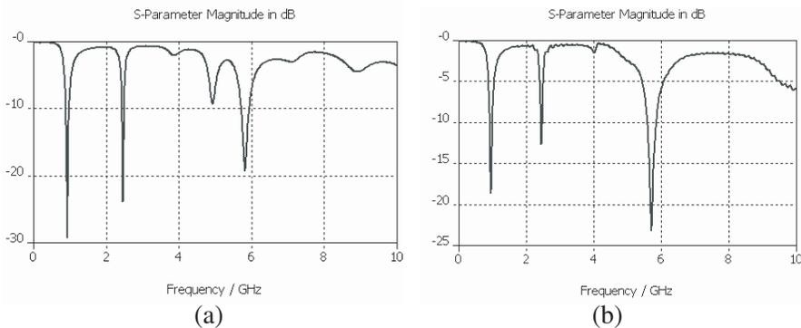
**Figure 2.** The simulated return loss of triple-band printed dipole antenna (a) design 1 ( $l_1 = 67.0$  mm,  $l_2 = 18.1$  mm,  $l_3 = 11.6$  mm,  $br = 4.5$  mm and  $h = 23.0$  mm) and (b) design 2 ( $l_1 = 77.3$  mm,  $l_2 = 18.1$  mm and  $l_3 = 10.6$  mm,  $br = 3.5$  mm and  $h = 23.0$  mm).
