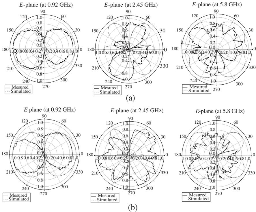
**Figure 7.** The simulated and measured radiation pattern of triple-band printed dipole antenna at 0.92 GHz, at 2.45 GHz and at 5.8 GHz (a) straight and (b) meandered.
