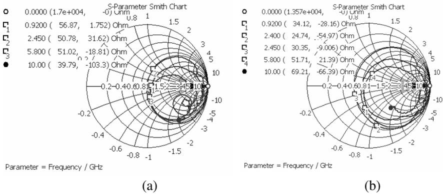
**Figure 3.** The simulated input impedance of triple-band printed dipole antenna for (a) straight and (b) meandered.
