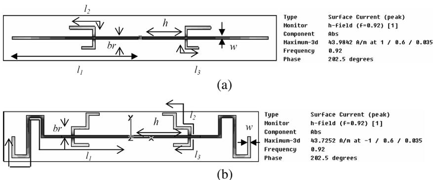
**Figure 1.** The structure of the designed triple-band printed dipole antenna and surface current at 0.92 GHz (a) straight (design 1) and (b) meandered (design 2).
