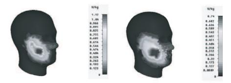
Figure 7. SAR distribution for the case of 1 g (left) and 10 g (right).
