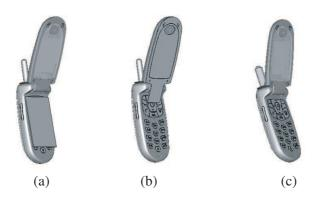
**Figure 3.** Three locations for R-card implementation, (a) case A: R-card covering keypad area, (b) case B: R-card covering LCD display and extending beyond antenna feed, and (c) R-card wrapping around the monopole antenna.
