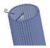
Figure 1. Geometry of a Cylindrical CNT Bundle composed of one circular shell.
