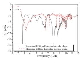
Figure 9. The comparison between simulated and measured of the reflection coefficient for embedded EBG.
