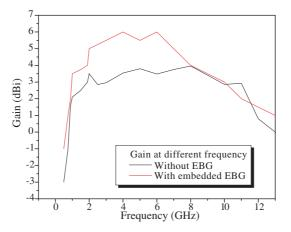
Figure 10. The MMPA gain without and with EBG structures.
