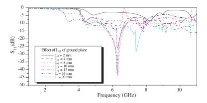
**Figure 3.** Effect of the antenna ground plane length  $L_q$ .
