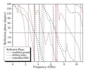
Figure 11. Reflection phase for MMPA without and with EBG structures.
