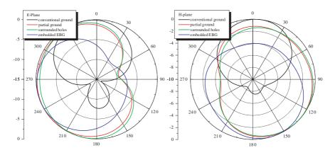
Figure 13. The measured E-plane and H-plane radiation pattern for MMPA at lower frequency (2.5 GHz).
