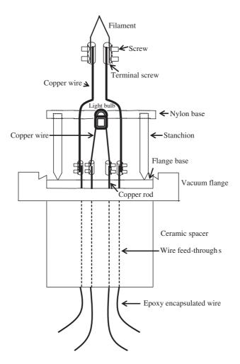
**Figure 7.** Filament mounting method using copper wires, screws and terminal screws.
