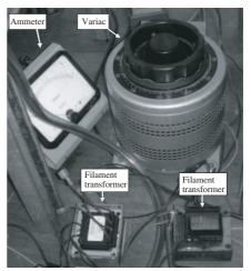
Figure 10. Electron gun circuit.
