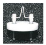
Figure 12. Photo of Thoria coated iridium filament.
