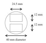
Figure 4. UBR100 standard waveguide flange.
