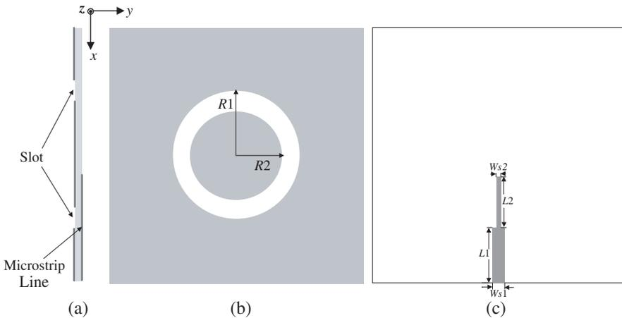
**Figure 4.** The geometry and coordinate system for the dualband slot antenna. (a) Substrate. (b) Slot in the groundplane. (c) Microstrip feedline.
