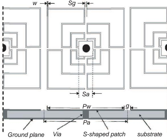
**Figure 1.** Geometry of the compact EBG cell.
