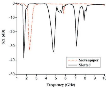
**Figure 3.** Comparison of  $S_{21}$  for sievenpiper and slotted EBG.
