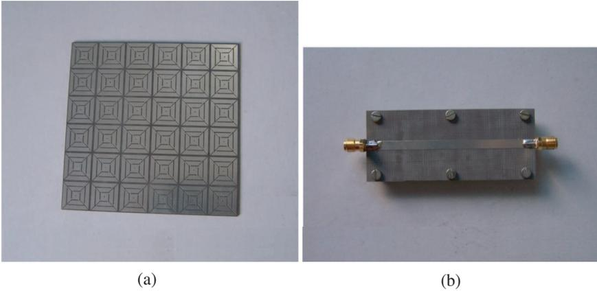
**Figure 6.** (a) Photograph of slotted EBG, (b) photograph of transmission line for slotted EBG.
