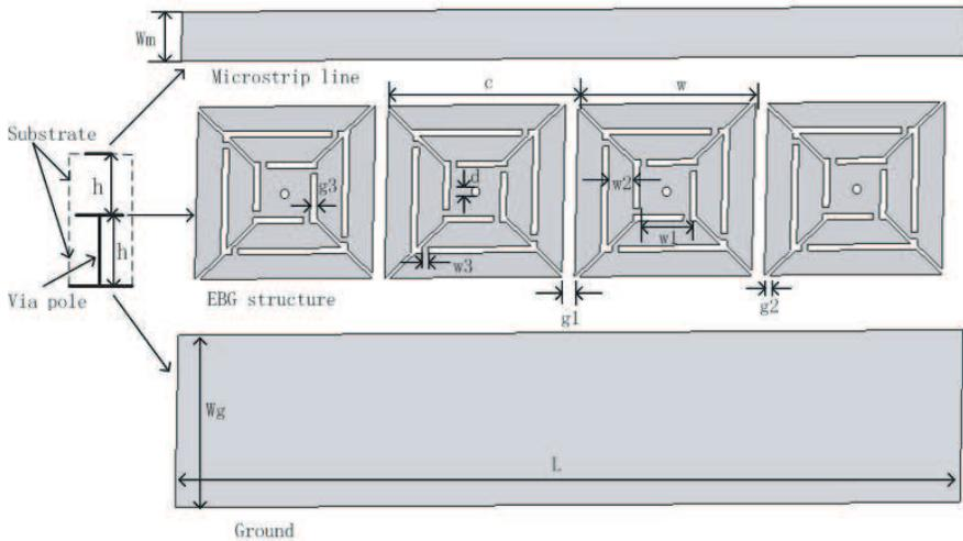
**Figure 2.** The model of transmission line for slotted EBG.
