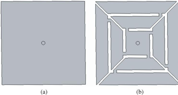
**Figure 1.** (a) Sievenpiper EBG structure, (b) slotted EBG structure.
