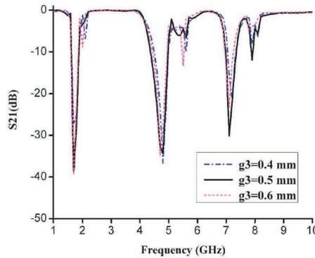
**Figure 5.** Comparison of  $S_{21}$  for different width of slots on trapezoids.
