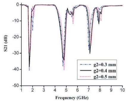
**Figure 4.** Comparison of  $S_{21}$  for different width of diagonal slots.
