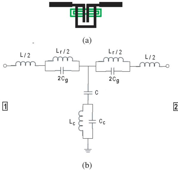
**Figure 3.** (a) The proposed loaded coupled transmission lines. (b) Its equivalent circuit model.
