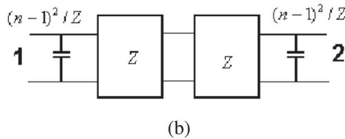
**Figure 1.** (a) The loaded coupled transmission lines [15]. (b) Its equivalent network model.
