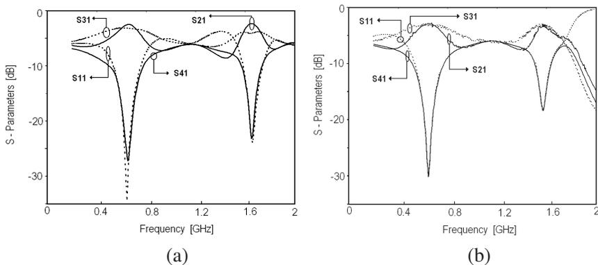
**Figure 6.** (a) The simulated and (b) measured  $S$ -parameters of the proposed dual-band BLC.
