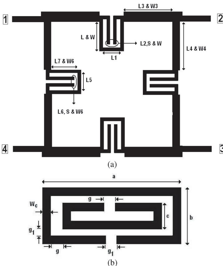
**Figure 4.** (a) Simulated layout of the proposed dual-band BLC. (b) The layout of used complementary split ring resonator (CSRR) with dimension of:  $L = 9.5$  mm,  $L_1 = 8.5$  mm,  $L_2 = 8$  mm,  $L_3 = 11$  mm,  $L_4 = 12$  mm,  $L_5 = 6.9$  mm,  $L_6 = 9$  mm,  $L_7 = 10.5$  mm,  $W = 2$  mm,  $W_3 = 2.91$  mm,  $W_4 = 1.715$  mm,  $W_6 = 1.2$  mm,  $S = 1$  mm,  $a = 12$  mm,  $b = 6$  mm,  $c = 4.4$  mm,  $W_c = 0.5$  mm,  $g = 0.3$  mm,  $g_1 = 1.2$  mm.
