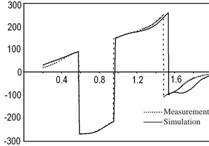
**Figure 7.** Phase difference between  $S_{21}$  and  $S_{31}$  in the dual-band BLC.
