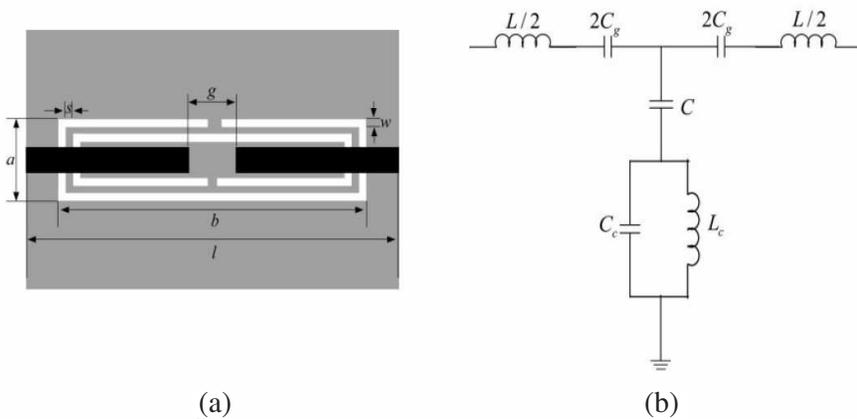
**Figure 2.** (a) and (b) the conventional dual-band BLC and its equivalent circuit model.
