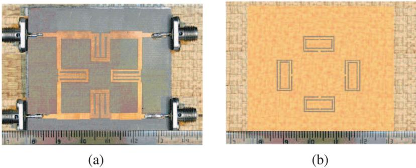
**Figure 5.** Photographs of the proposed dual-band BLC: (a) top face; (b) bottom face.
