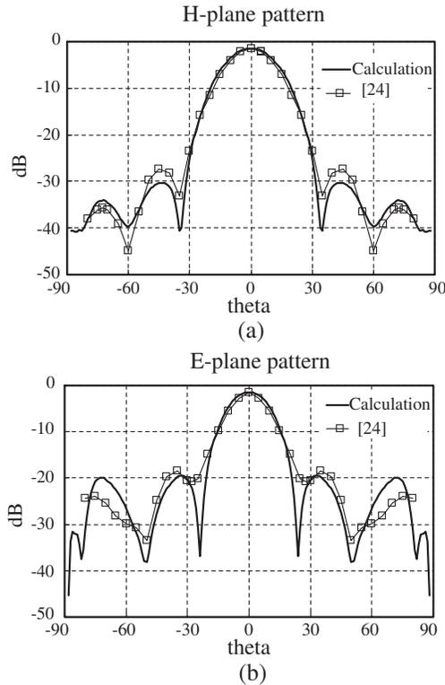
**Figure 3.** Radiation pattern of a radome enclosed antenna, which has a circular aperture in a hemi-spherical shell radome.
