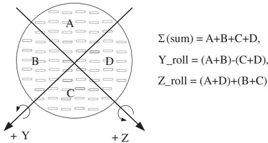
**Figure 7.** Bore-sight error voltage calculations. (a) BSE voltages calculated with the antenna rotated along the  $y$ -roll angles. (b) Aperture distributions and rotation angles.
