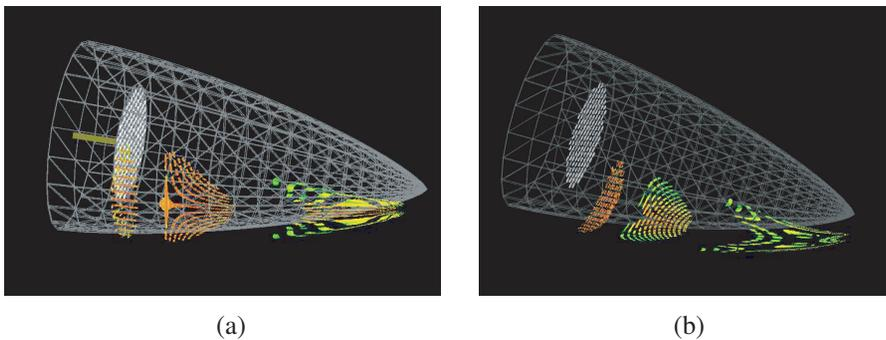
**Figure 5.** Projected current formed on a curved surface seen at the angle of 80 degrees from the observation points on the  $H$  and  $E$  planes. (a) A projected current distribution seen from a point on the  $H$ -plane. (b) A projected current distribution seen from a point on the  $E$ -plane.
