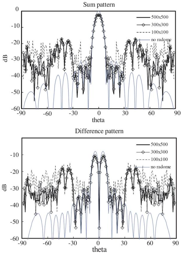
**Figure 6.** Variations of the radiation patterns ( $H$ -plane) with grid sizes. The projection plane is a square with each side  $40\lambda$  long. “ $300 \times 300$ ” means that the square is divided into  $300 \times 300$  squares with sides  $0.13\lambda (= 40\lambda/300)$  long.
