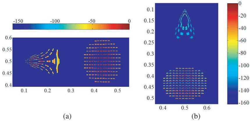
**Figure 4.** A strength map of the projected current of a monostatic antenna is drawn on a log scale normalized to the maximum current density. The numbers on the axes are scaled values to the maximum dimensions of the projection plane. (a) Projected current distribution seen from an observation point on  $H$ -plane. (b) Projected current distribution seen from an observation point on  $E$ -plane.
