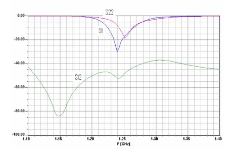
Figure 4. Return loss at L-band frequencies.
