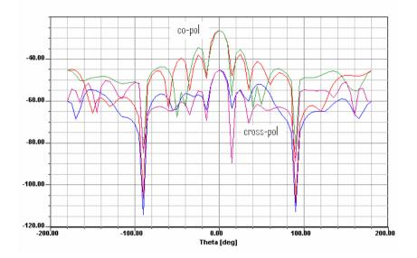
Figure 6. Radiation pattern for C-band with only port 1 excited.
