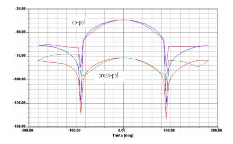
Figure 9. Radiation pattern for L-band with only port 2 excited.
