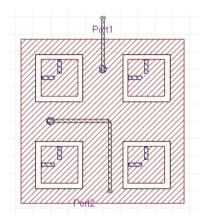
Figure 3. L-band perforated patch overlaid on top of C-band patches.
