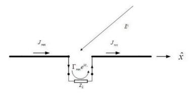
Figure 2. Feed port reflection of element with load  $Z_L$  in array.
