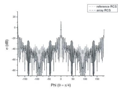
Figure 6. Comparison of the two different solutions for the array RCS with  $\theta = \pi/4$ .
