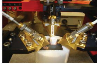
Figure 5. Circulator under test using three probes system; two probes are connected to the VNA and the third one (central one) is connected to an adapted load.
