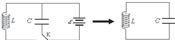
Figure 1. Scheme for LC electromagnetic oscillation.
