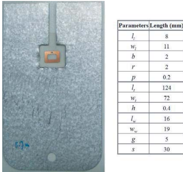
Figure 10. The photograph and physical dimensions of the implemented WinTag antenna.
