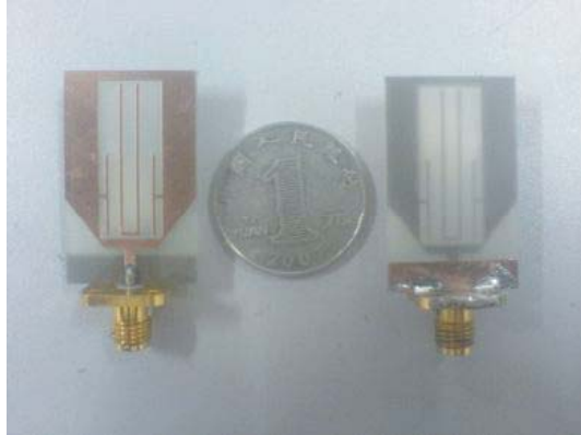
Figure 2. Photograph of the proposed antenna.
