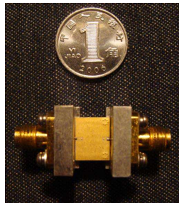
Figure 4. Photograph of 16\lambda_g multilayer LTCC delay line with the test fixture.
