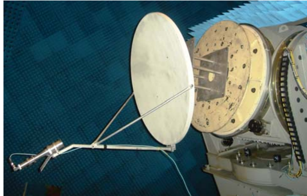
Figure 7. The offset reflector and a circularly polarized tri-mode matched feed under test at Compact Antenna Test Range (CATR).
